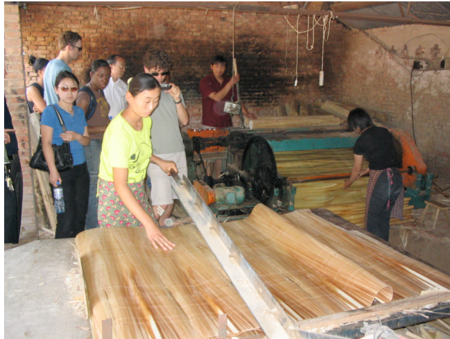
Fig. 3: A local woman lays out wood veneer that has just been processed at a small scale wood-products manufacturing enterprise in Heze, Shandong. In the far right corner, another woman runs a lathe to continue veneer production. Local poplar logs were used in this process.
