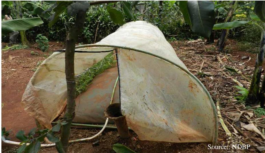
Figure 18: Flex bag biodigester (Rwigema, 2015)
